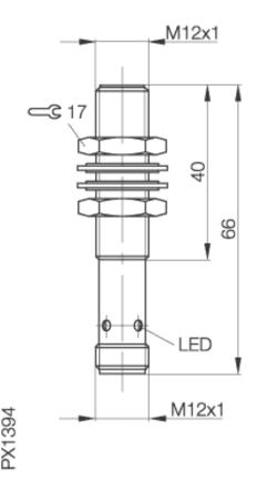
**Inductive Sensors BES M12EL-PSC20B-S04G-M01** M12x1 x 66 normally-open Sn=2mm shielded
